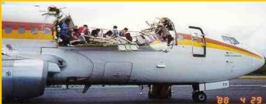
An example of an incident that may have been prevented by SHM is the 1988 Aloha Airlines Flight 243 where undetected fatigue cracks led to a weakened structure. 20 minutes into a flight, at 24,000 ft altitude, the roof of the aircraft ripped off, injuring 65 people and killing one.
