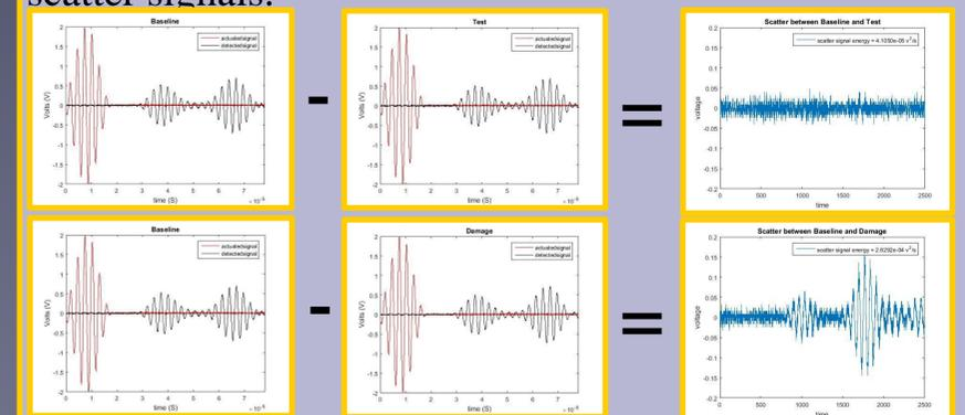
The calculated signal energies indicate a greater change in the signal when damage is present.
