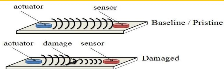
A typical setup, as shown in the picture above, consists of a piezoelectric actuator that generates ultrasonic waves, which propagate through the structure, and a piezoelectric sensor that detect the waveforms. Damage causes changes in the waveforms.
