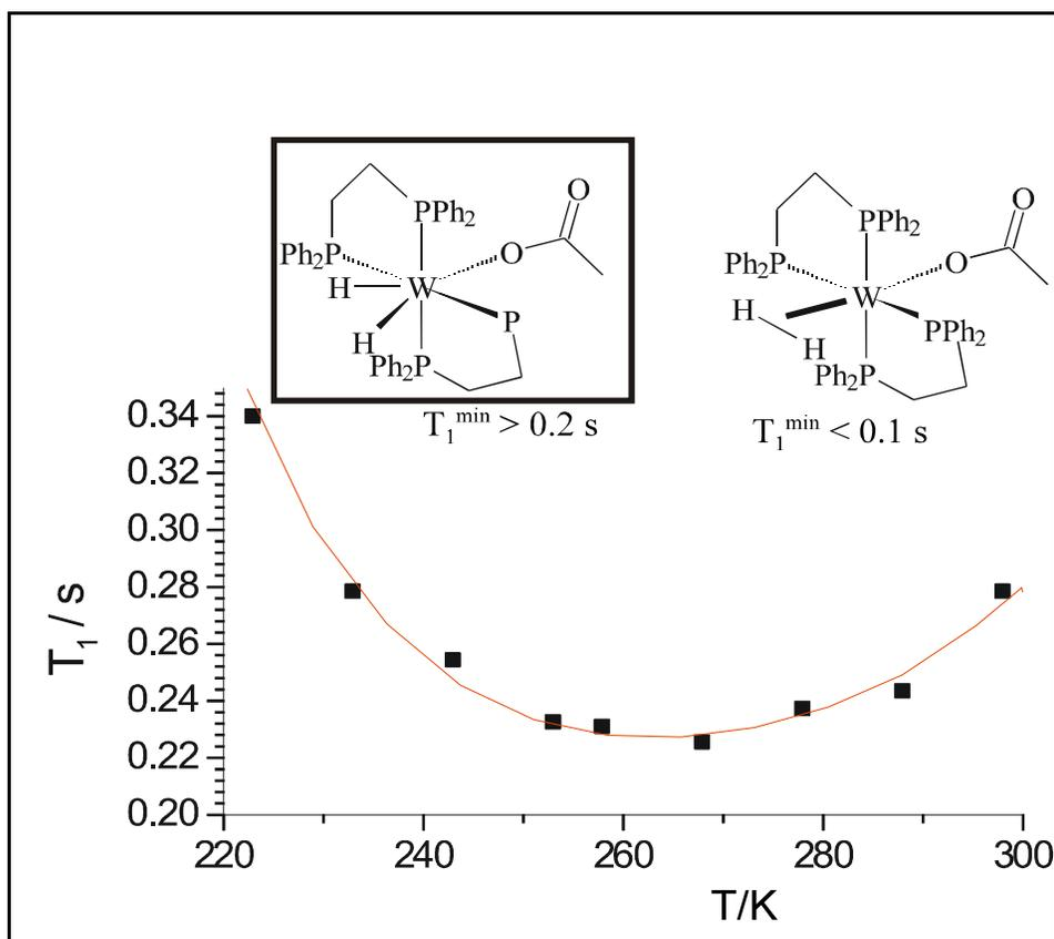
Use of  $T_1$  measurement to distinguish two possible structures: The hydride H-H distance in the dihydride complex is considerably longer than in the dihydrogen complex, resulting in different predicted values for  $T_1^{\min}$ . The experimental  $T_1^{\min} = 0.23$  s and thus indicates the presence of the dihydride complex.
