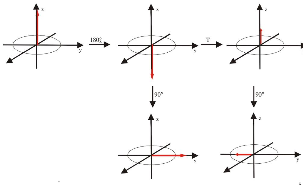
The  $180^\circ$  pulse place the magnetization along the  $-z$  axis. During the waiting time  $T$  the magnetization will relax back towards its equilibrium value. The  $90^\circ$  pulse will then convert the
