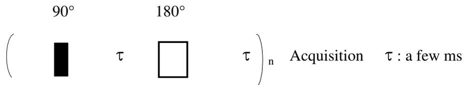
As for  $T_1$  measurements several spectra with different delay times are obtained and the dependence of the signal intensity on the delay time is monitored. In this case one varies the number of cycles  $n$  and the total delay time is  $T = 2n\tau$ . As inhomogeneity is refocused the signal decay depends only on  $T_2$ :
