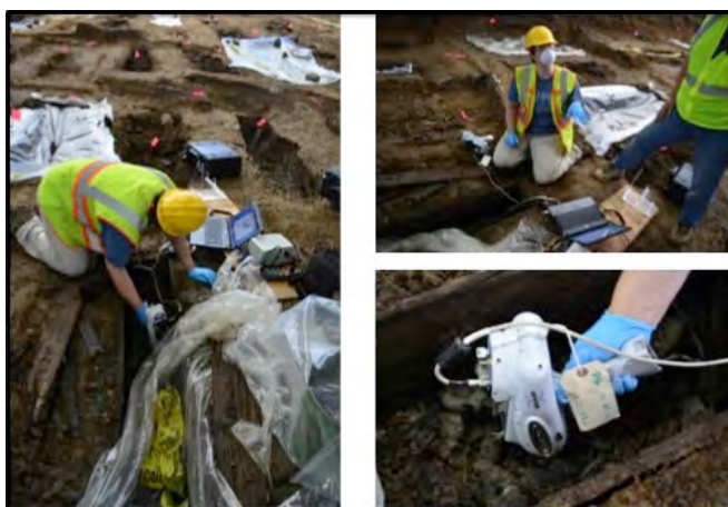
Figure 4.48. pXRF field analysis of soils, (UWM photo on file, UWM-ARL).
