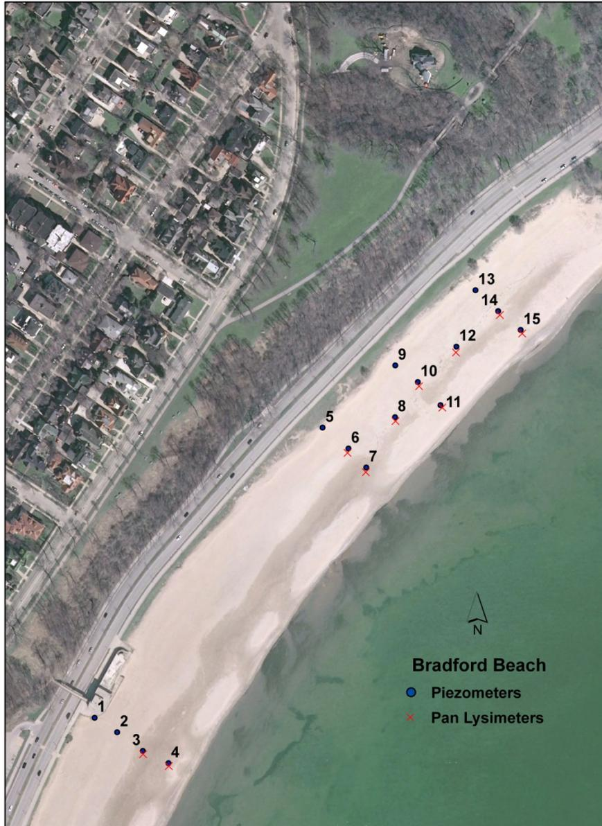
Figure 5- Sampling sites of subsurface water (groundwater sampled at the piezometers and runoff infiltrating through the sand sampled at the pan lysimeters)
