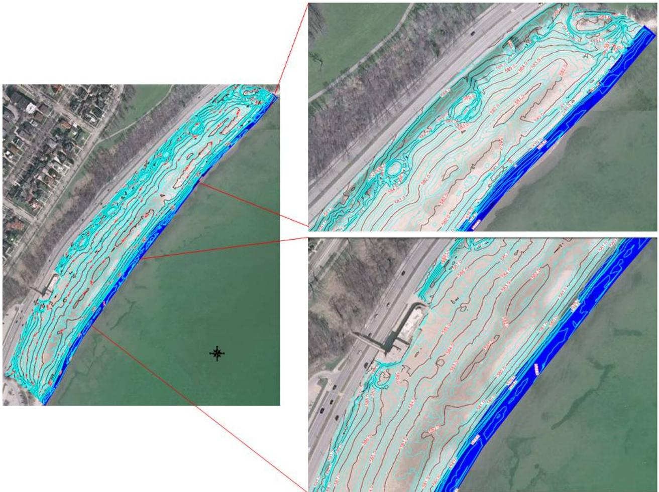
**Figure 10-Topographical survey of Bradford Beach in April 2010. Note that after the winter time and beginning of Spring; again the region with the largest deepest depression (581 ft) is located on the northern part of the beach. Note that the swash zone (dark blue area) was also surveyed in April.**
