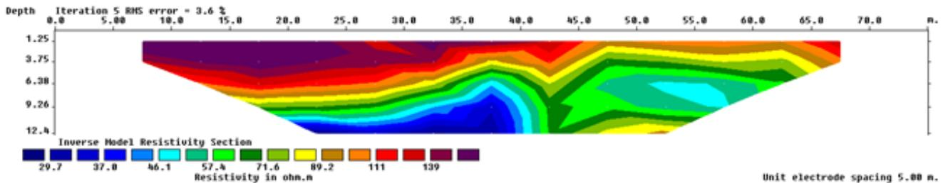
Figure 35-Resistivity profile (pseudosection) with 5 meter spacing. The graph is interpreted layer parameters. It shows higher resistivity to the south and lower resistivity at depth. This profile is sensing to approximately 6 m depth at the center.
