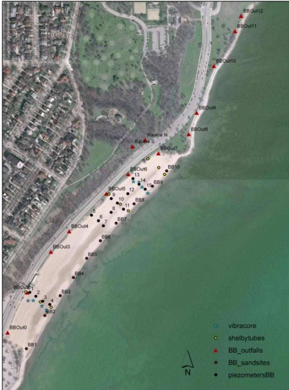
Figure ES- 2- Sampling sites. The yellow circles show the sites where sand cores were collected with Shelby tubes in 2007, the blue stars show the transects of sand cores collected in 2009 with a vibracore, the black circles show where piezometers were installed in October 2009, the red triangles show where the stormwater outfalls are located and the red circles show where the berm surface sand sites are located. Please note the region of wet sand along the beach.
