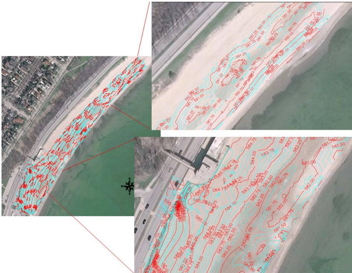
**Figure 9-Topographical survey of Bradford Beach in November 2009. Note that a) the overall southern part has higher ground elevation than the northern part and b) the deepest depressions (swale) are located on the wet area that is observed along the beach (581.50 ft on the southern part and 581.00 ft on the northern part).**
