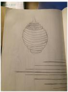
Since the urban Ash wood we were given isn't able to be made into a flexible curve, I designed a topographic shape instead. It's important that the bees have small openings to travel into, but are guarded off against predators at the same time.
