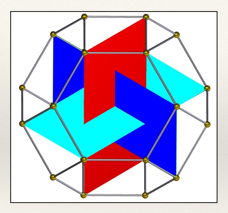
A convex Icosahedron showing the internal rectangles forming the points.
