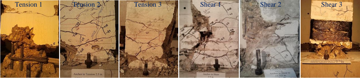
Figure 4.38: Summary of NEES-Anchor tests of reinforced anchors in plastic hinge zones
