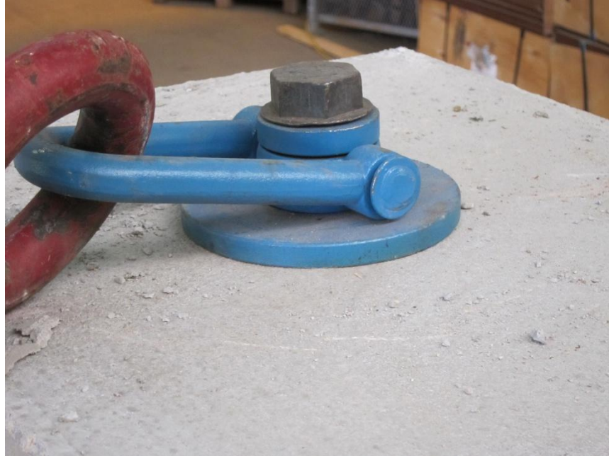
Figure C.16: Photo of Lift Point on Structural wall
