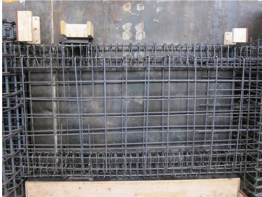
Figure C.12: Photo of Wall Specimen Reinforcing
