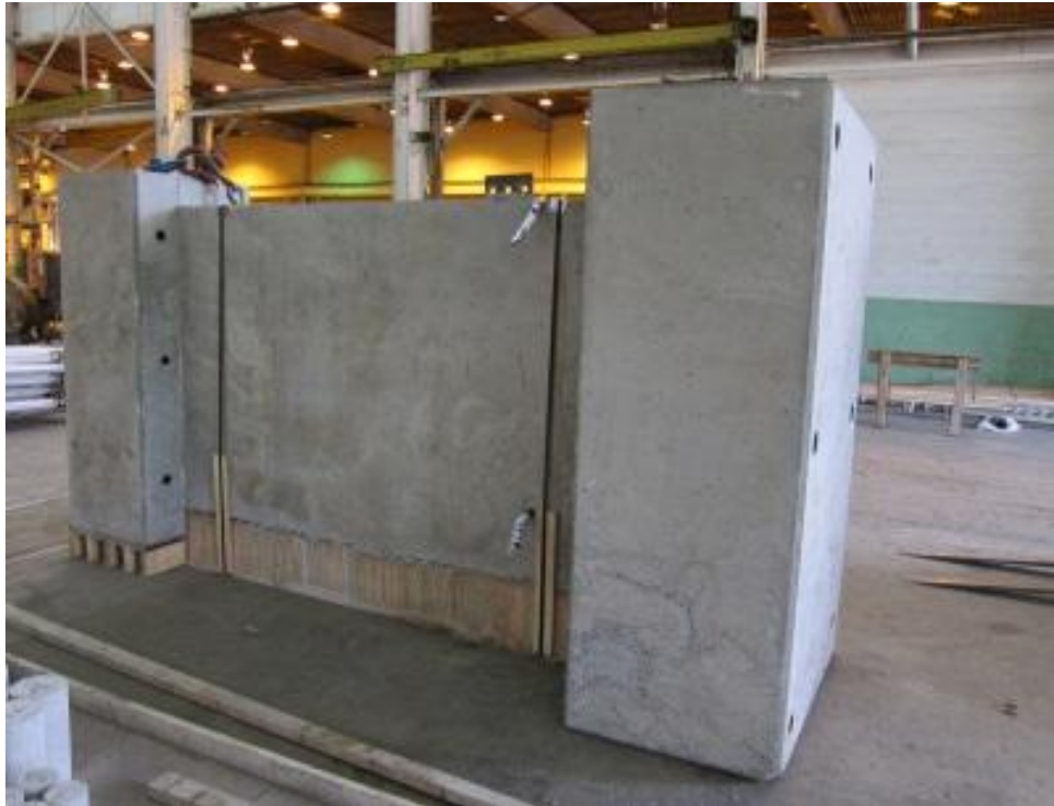
Figure C.9: Photo of Wall Specimen Right After Concrete Placement
