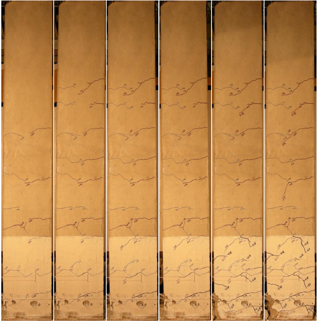
(a) \pm 0.58 in. (b) \pm 1.12 in. (c) \pm 1.66 in. (d) \pm 2.20 in. (e) \pm 3.28 in. (f) \pm 4.9 in. Figure A.7-Crack development after all loading cycles (T2)
