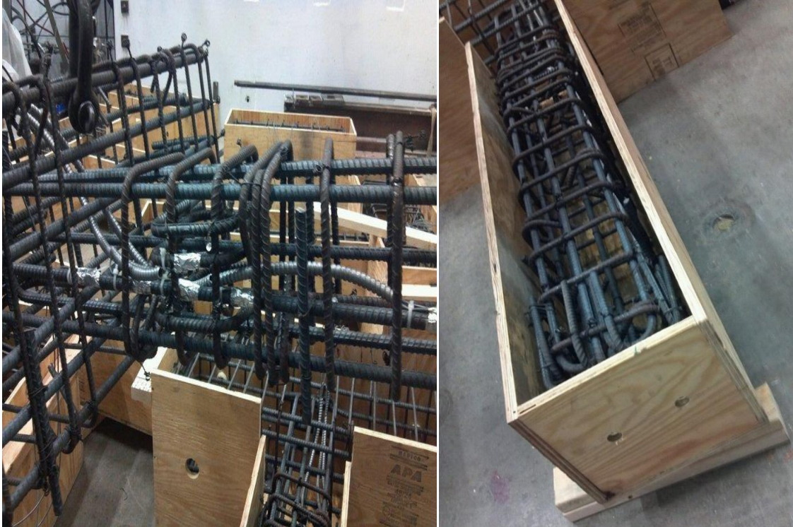
Figure 3.4: Reinforcing steel cage of Phase V specimens
