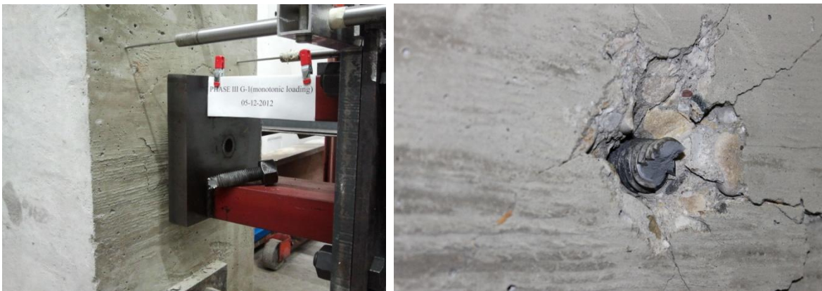
Figure 5.26: Failure of 1.0-in. anchors with Type G reinforcement under monotonic tension
