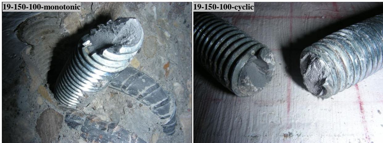
Figure 5.13: Typical fractured shape of 3/4-in. anchor bolts
