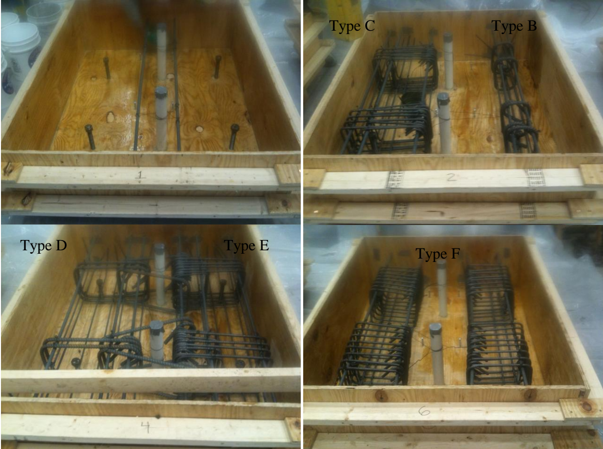
Figure 4.8: Anchor tension reinforcement in Phase III tests
