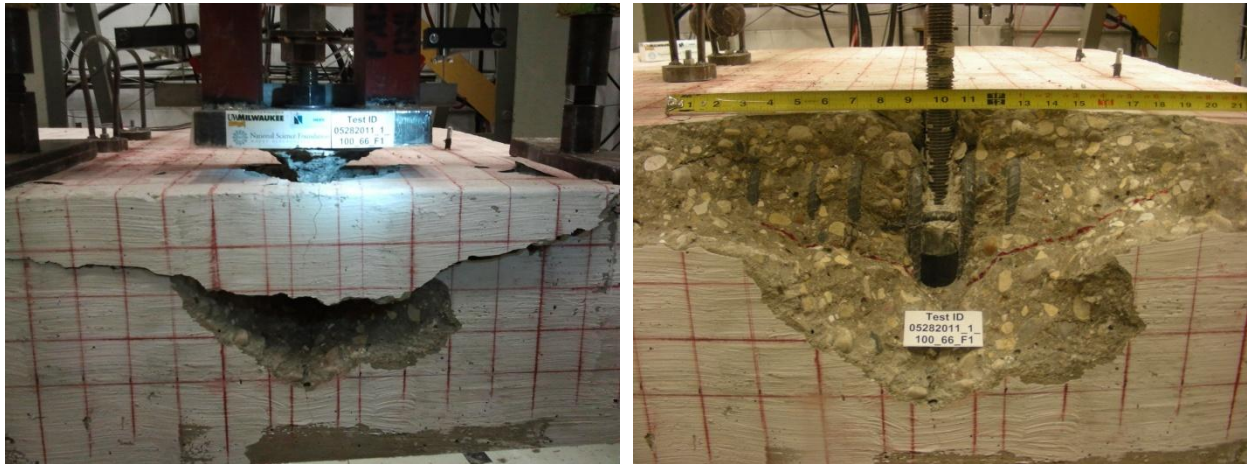
Figure 5.24: Failure of 1.0-in. anchors with Type F reinforcement under monotonic tension
