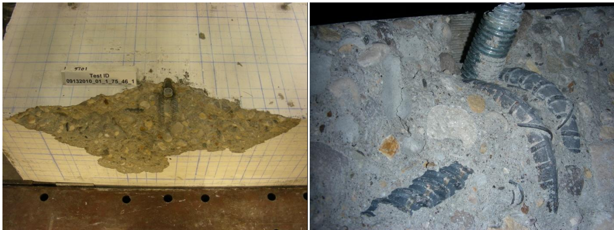
Figure 5.2: Concrete cover pushed off during shear tests of 3/4-in. anchors
