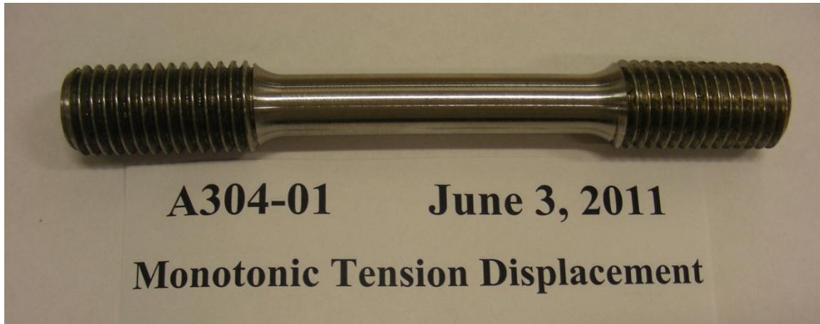
Figure 5.43: Standard 0.5-in (12.7-mm) diameter coupon of A304 anchor rods
