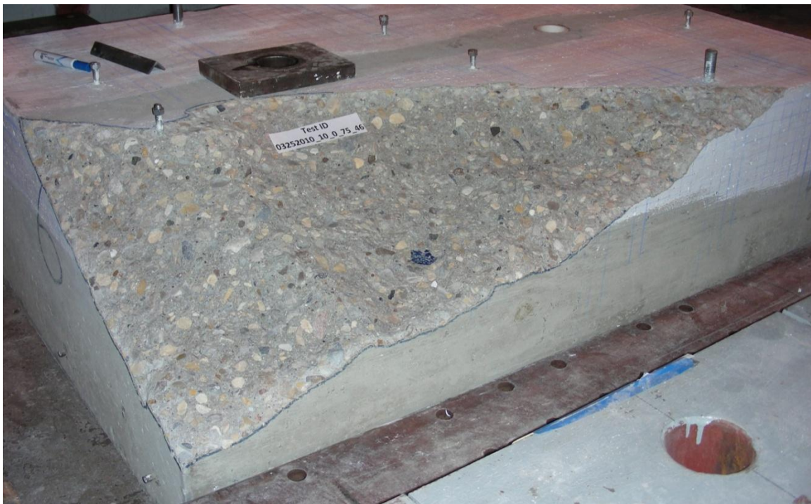
Figure 4.15: Tension breakout cone interference ( d_a = 0.75'' , h_{ef} = 6'' , c_{al} = 4'' )
