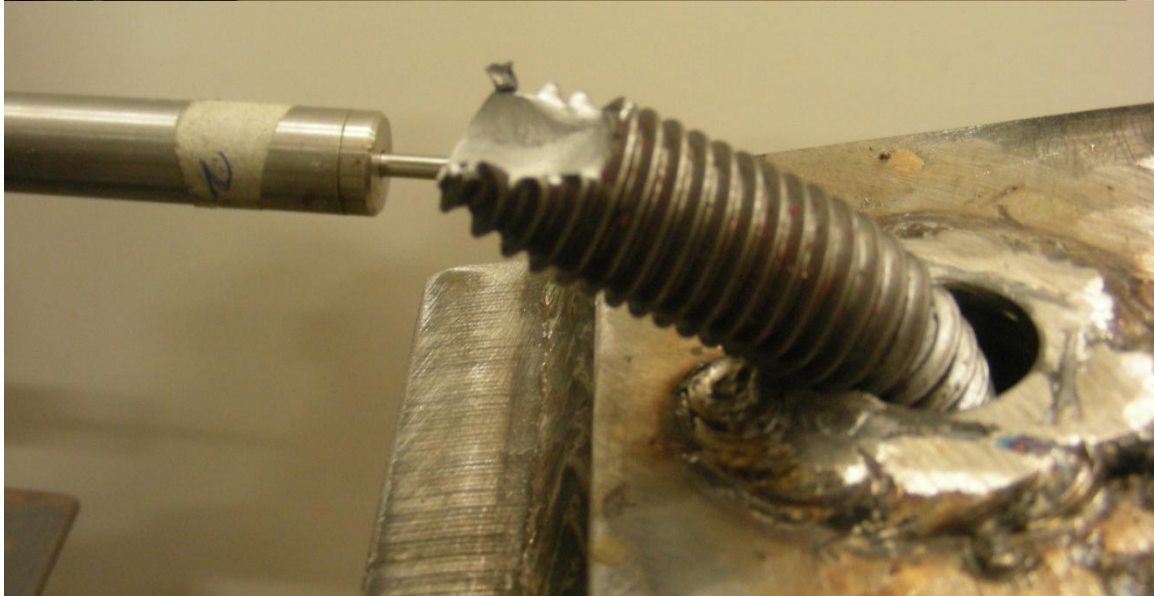
Figure 5.40: fractured rods in double-shear tests
