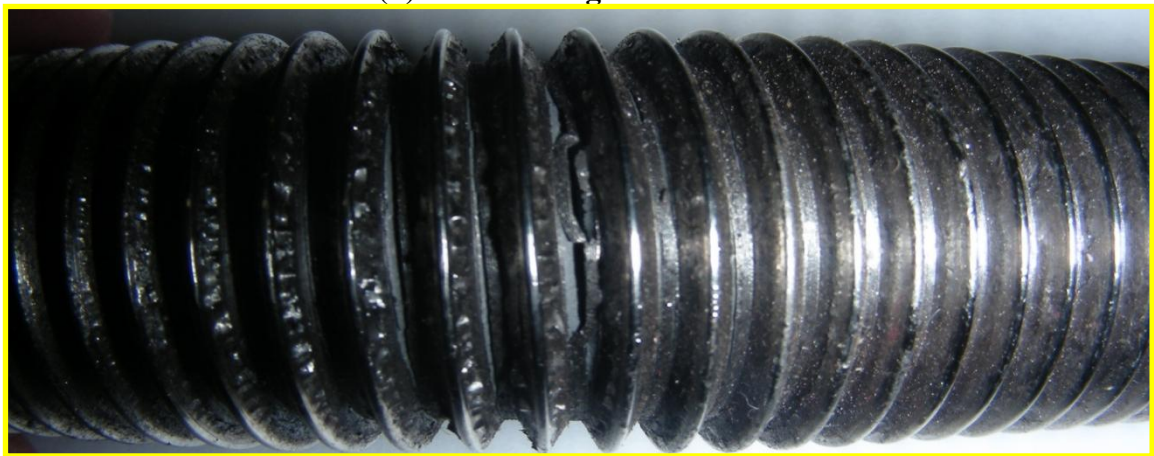
(c) flexural crack opening Figure 5.14: A193-4da-MD
