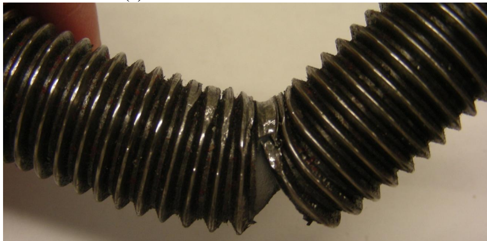
(b) local bearing deformation
