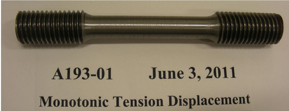
Figure 5.2: Standard 0.5-in (12.7-mm) diameter coupon of A193 anchor rods
