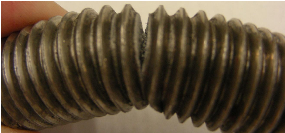
(b) flexural crack opening Figure 5.59: A304-2da- RL
