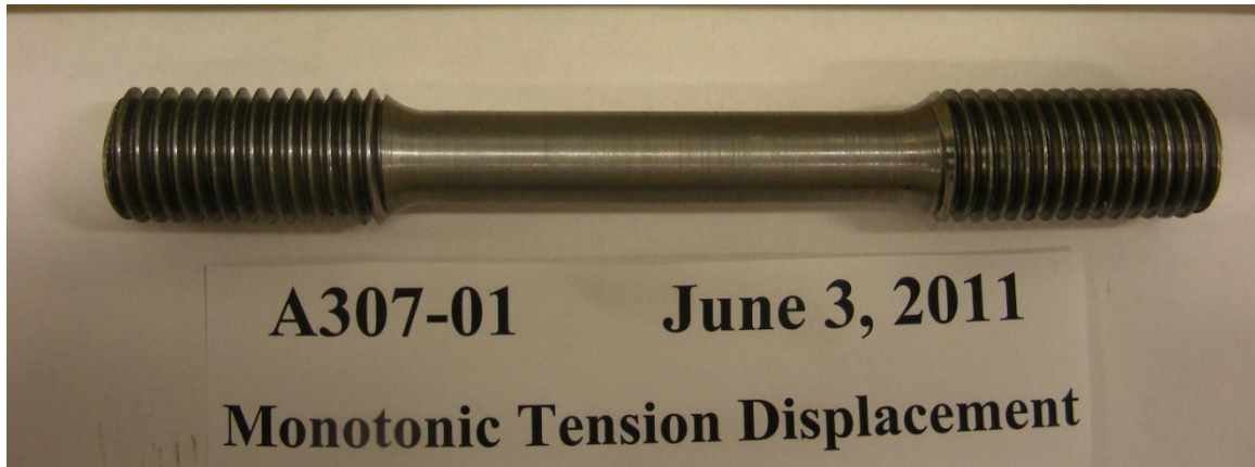
Figure 5.23: Standard 0.5-in (12.7-mm) diameter coupon of A307 anchor rods
