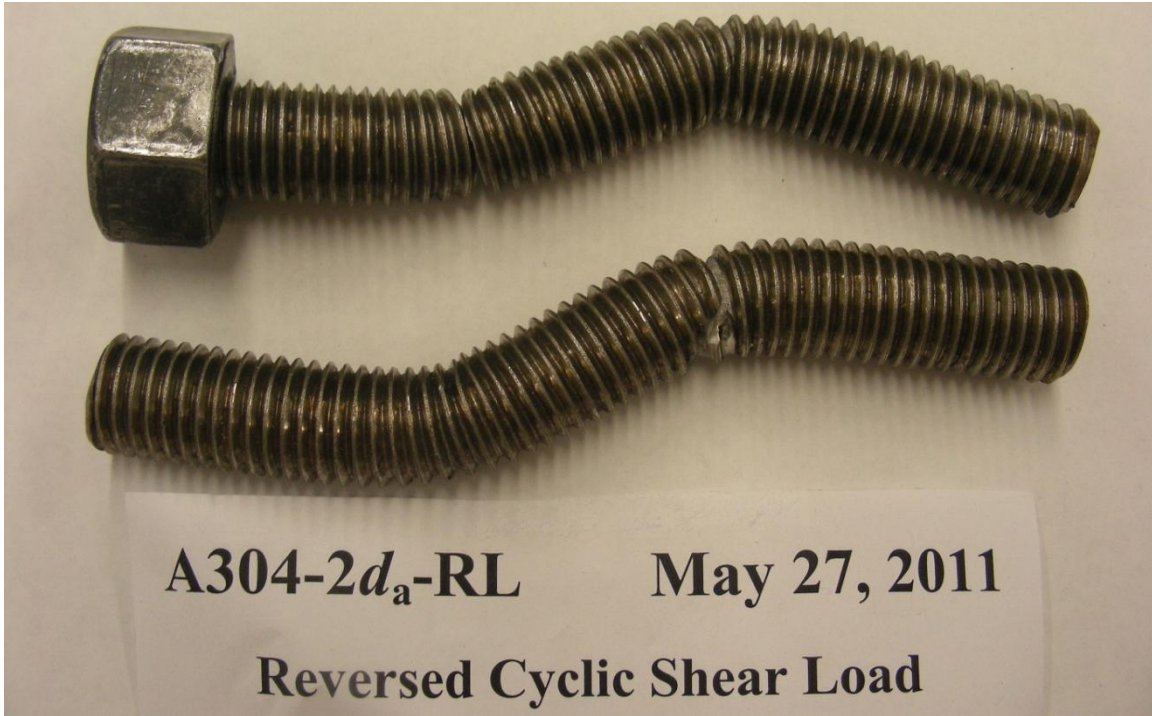
deformation of two anchor rods
