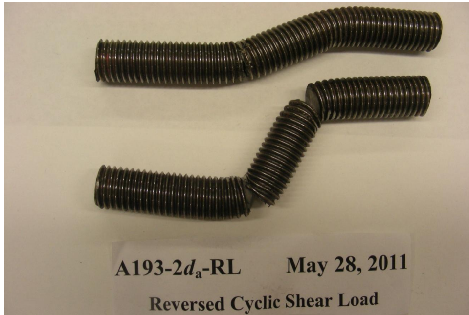
(a) deformation of two anchor rods
