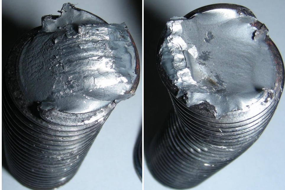
(a) one side of the fractured rod
