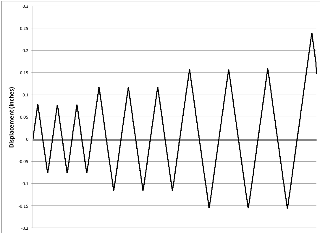
Figure 3.11: Cyclic shear loading profile (Actuator displacement)
