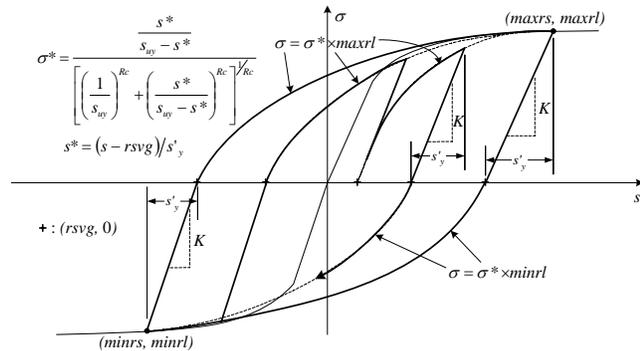
Figure 4. Hysteresis rule for the bar stress vs. loaded end slip of fully anchored bars into footings.
