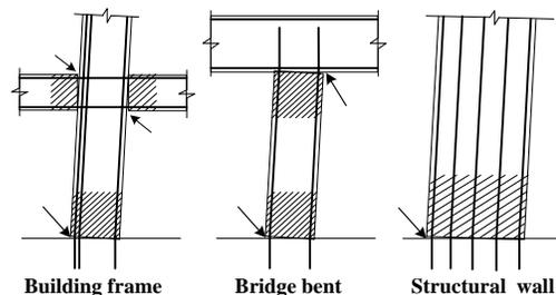
Figure 1. Typical inelastic regions in well-designed concrete structures
