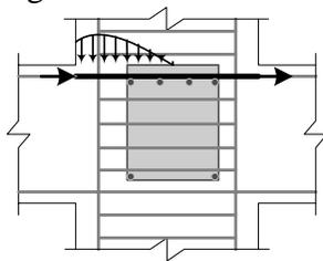
*Beam bars in building joints*
