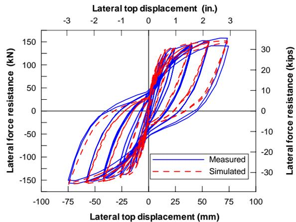
Figure 7. Measured vs. simulated response of RW2.
