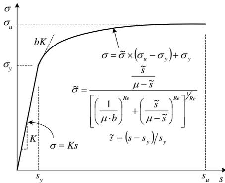
Figure 3. Bar stress vs. loaded end slip for fully anchored reinforcing bars into footings.
