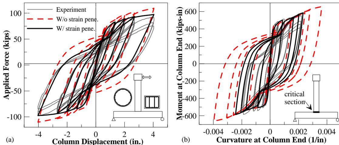
Figure 8. Comparison of experimental and analytical results for T-joint specimen IC1
