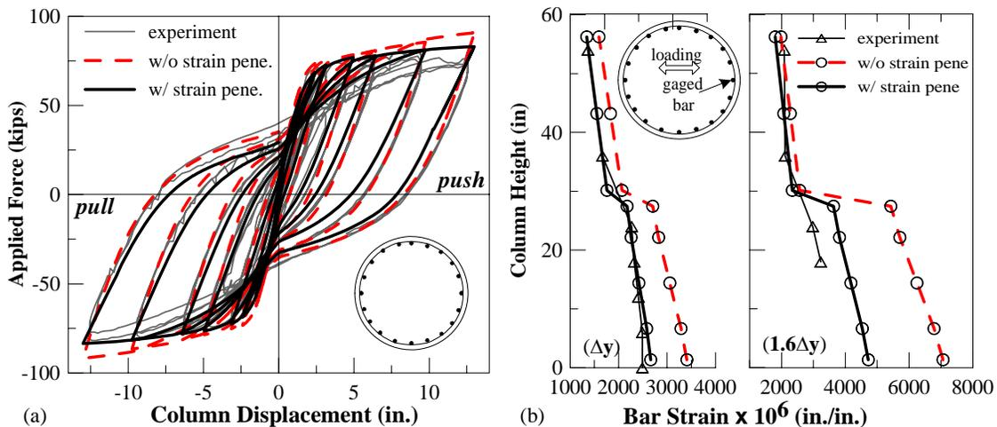
Figure 5. Comparison of experimental and analytical results for a cantilever column
