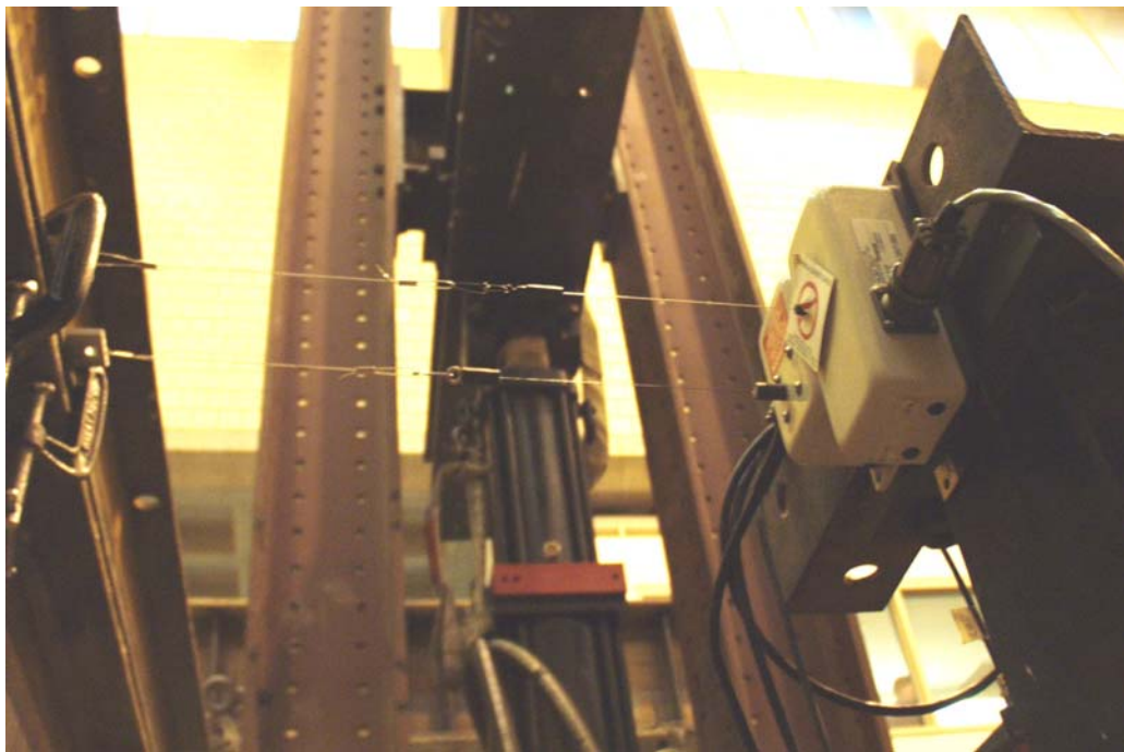
Figure A7.5 Connection of the velocity and displacement transducers from a reaction frame to the test structure (EFT)
