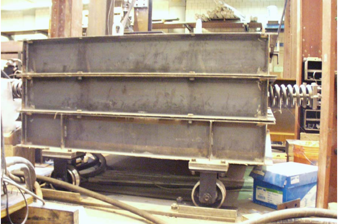
Figure A4.1 Three steel frames filled with concrete atop four caster wheels
