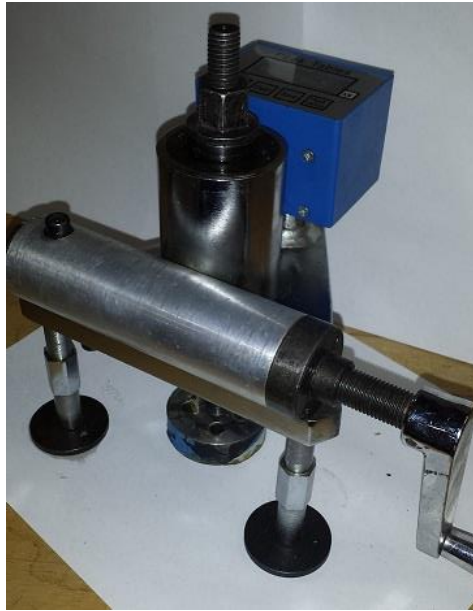
Figure 25. Pull-out test device.
