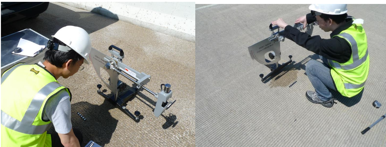
Figure 29. Friction testing using BPT.
