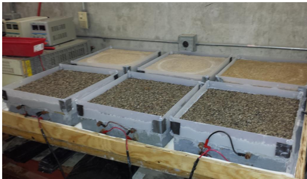
Figure 8. Accelerated corrosion setup.
