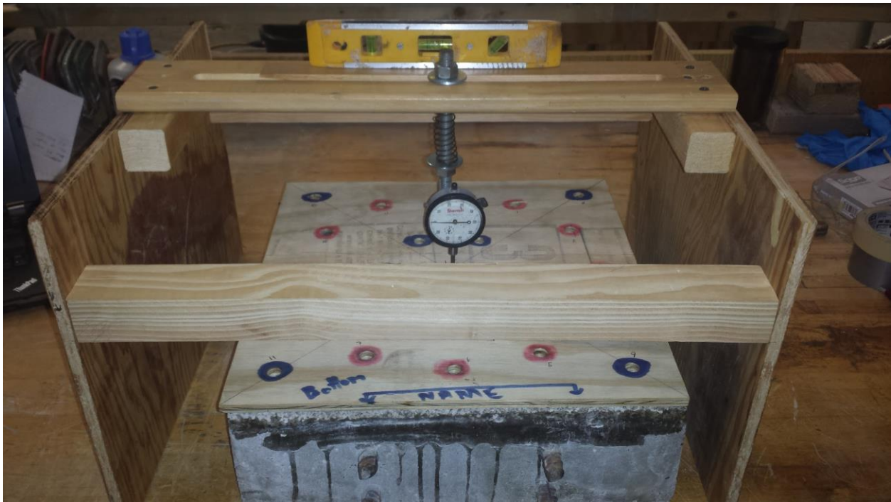
Figure 26. Measurement of the depth of surface groove (rut) through a dial gage at measurement points defined using a wooden template.
