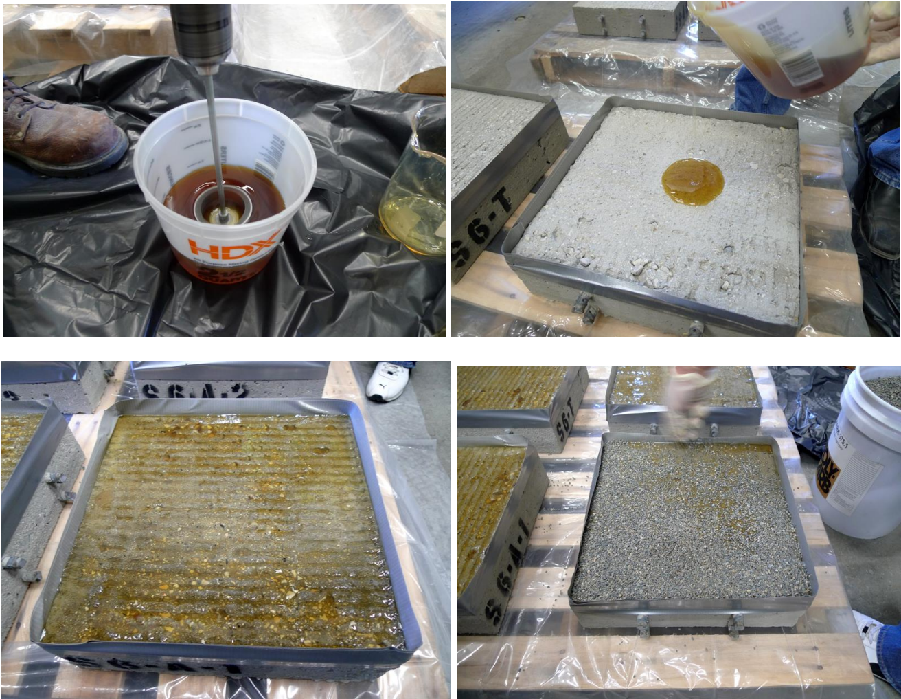
Figure 4. Placement of thin polymer overlay on test specimen.
