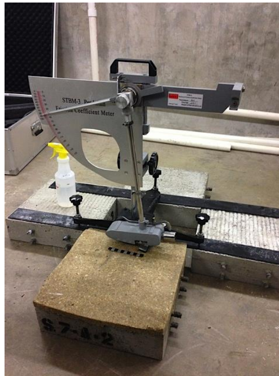
Figure 20. British Pendulum Tester used on specimens prior to exposure tests.
