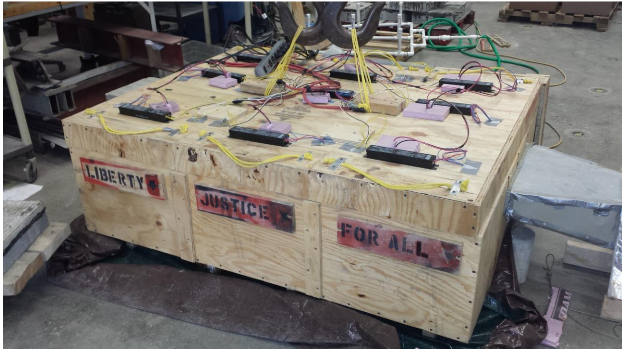
Figure 14. Manual HURA test box.
