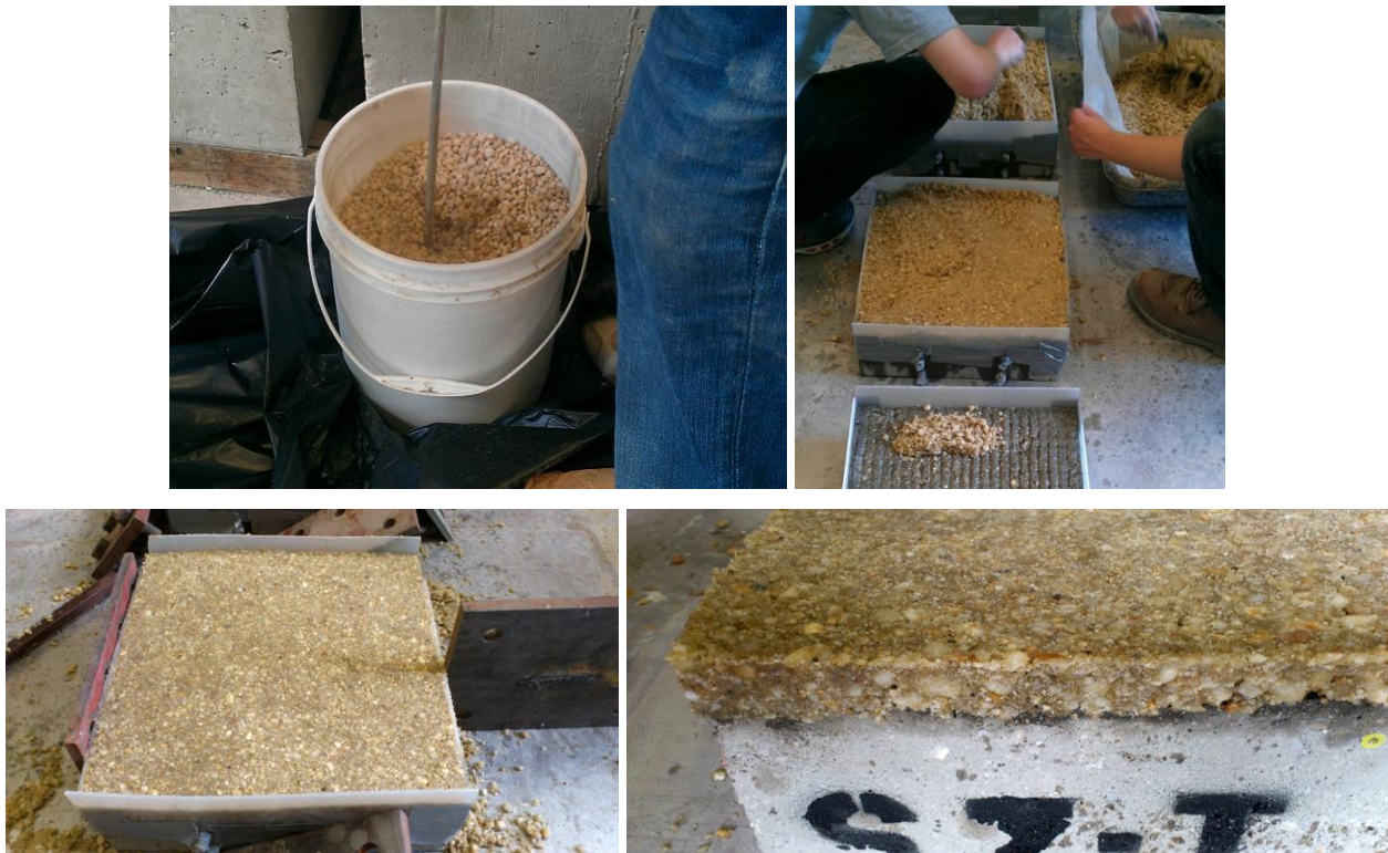
Figure 6. Pre-mixed polyester overlay system (S7) placement.
