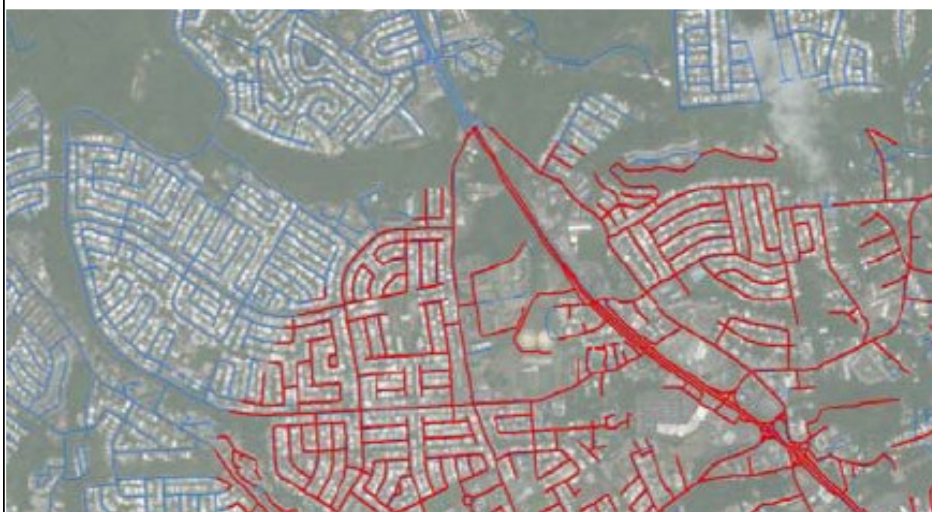
3) Manually edit edgework by stretching/trimming vertices
