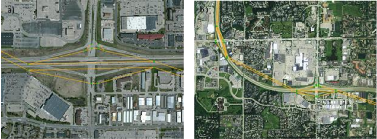
Figure 2.2. STN representation (orange lines) of a typical divided highway with exits, (a) close up of off ramps showing turn lanes, (b) shows a larger image of STN link representation.
