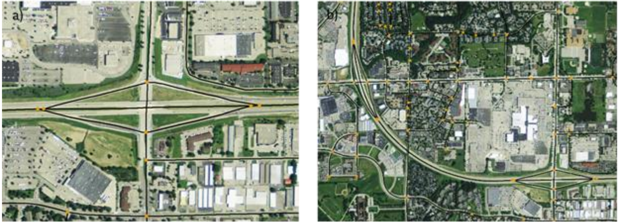
Figure 2.3. WISLR representation (black lines) of typical divided state highway, (a) close up of exit, (b) larger image showing cartographic nature of WISLR.
