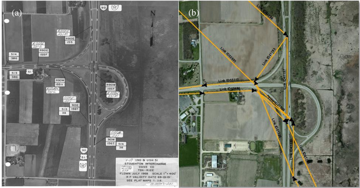
Figure 3.1. RP diagram (a) detailing roadway types and route names associated with STN links (b) at the interchange.
