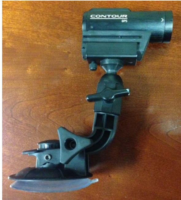
Figure 3.2. GPS-enabled camera that can be set to take pictures at a time interval.
