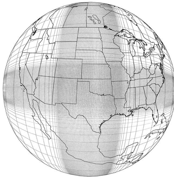
Figure 10. An example of a stretched horizontal grid. In this example, the full limited-area model domain is 353 x 415 grid points, with the centermost 240 x 323 grid points having uniform horizontal resolution. The horizontal grid spacing decreases by 10% per each model grid length as one moves from the periphery of the limited-area domain, where it is identical to that of the global model used to initialize and provide lateral boundary conditions to the simulation ( 2^\circ ), to the center of the limited-area domain, where it is 0.04^\circ . Figure obtained from Yeh et al. (2002, Mon. Wea. Rev. ), their Fig. 6.
