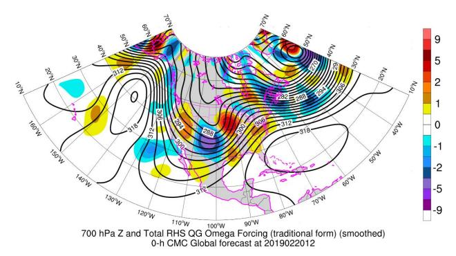
**Figure 5**. 700 hPa geopotential height (contours every 6 dam = 60 m) and the sum of the forcing terms depicted in Figs. 2 and 4 ( $x10^{-12}$  Pa m<sup>-2</sup> s<sup>-1</sup>, shaded per the color bar at right) from the 0-h CMC analysis at 1200 UTC 20 February 2019.
