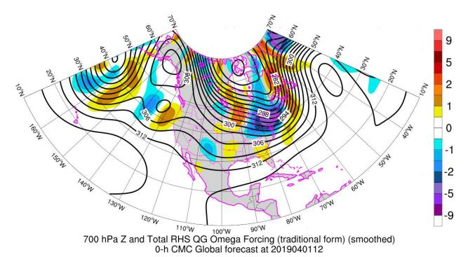
**Figure 5**. 700 hPa geopotential height (black contours every 30 m = 3 dam) and total forcing from the right-hand-side of the quasi-geostrophic omega equation (shaded per the color bar at right, with positive values indicating forcing for ascent; units:  $x10^{-12}$  Pa m<sup>-2</sup> s<sup>-1</sup>) at 1200 UTC 1 April 2019, obtained from https://inside.nssl.noaa.gov/tgalarneau/real-time-qg-diagnostics/.
