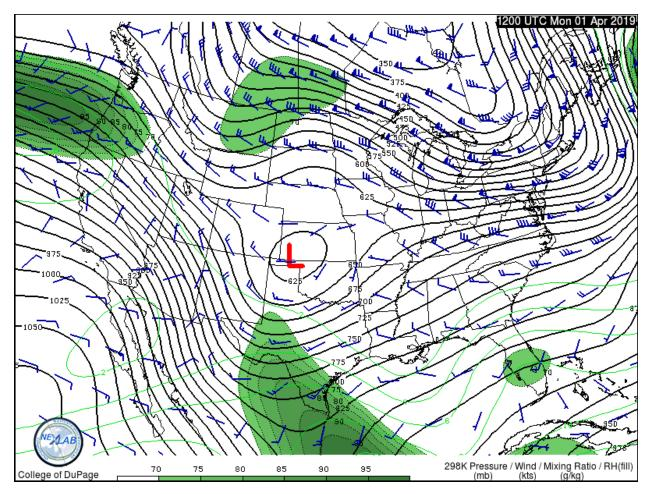
**Figure 4**. 298-K pressure (black contours every 25 hPa), wind (barbs; half-barb: 5 kt, full barb: 10 kt, pennant: 50 kt), mixing ratio (green contours every 1 g kg<sup>-1</sup> starting at 2 g kg<sup>-1</sup>), and relative humidity (shaded in % per the color bar) at 1200 UTC 1 April 2019, obtained from the College of DuPage (https://weather.cod.edu/analysis/).
