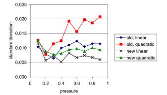
Figure 6. Standard deviation for different pressure levels during 3s intervals. Overall variability is better for the new hardware and the linear mapping.
