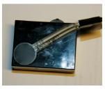
Figure 11. Shake device for vibrotactile feedback with FSR on top.
