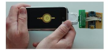
Figure 1. Sandwich prototype for two-sided multitouch sensing with continuous pressure input.
