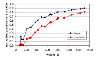
Figure 3. Combined characteristic of FSR response curve and voltage divider.
