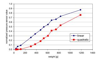
Figure 5. Combined characteristic of FSR response curve and opampbased circuit.
