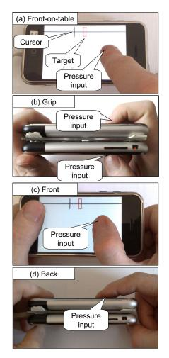
Figure 7. Device poses tested for handheld pressure input: (a) index finger on front, device resting on table (baseline); (b) grip with thumb and index finger; (c) thumb on front; (d) index finger on back. Changing pressure moves the cursor on the horizontal line. The red rectangle indicates the target pressure and target width.
